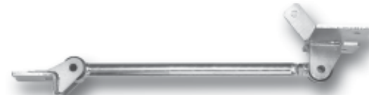
A CADMIUM-PLATED RSS ANTI-SWAY BAR bolted in place. Most installations take about the same amount of time as shock absorbers.
